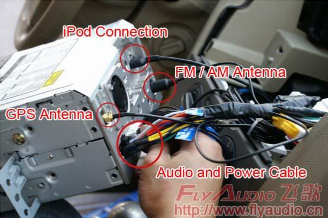
12.connect the tidy cable to the new head unit in place
