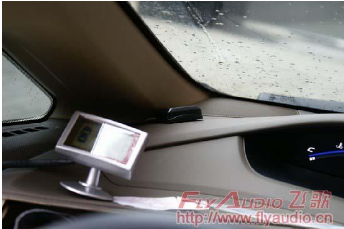
31.Position GPS antenna properly
