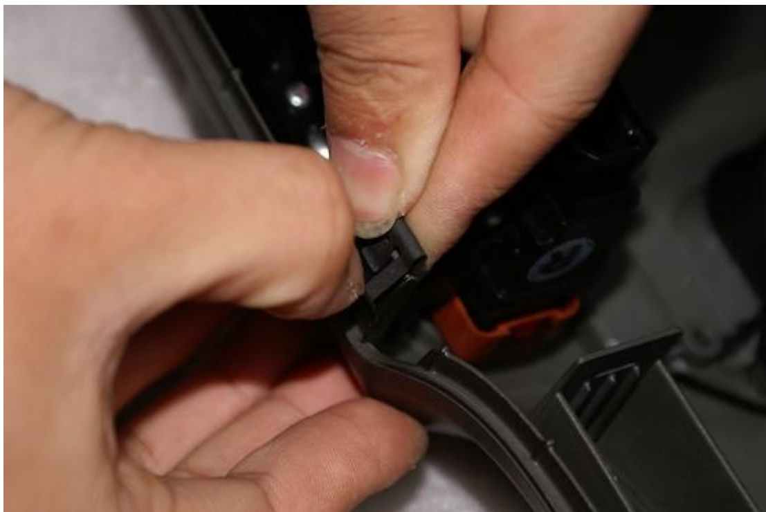
28.Install buckle on special panel.
