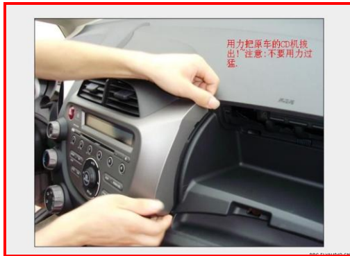
11: Remove the factory unit
