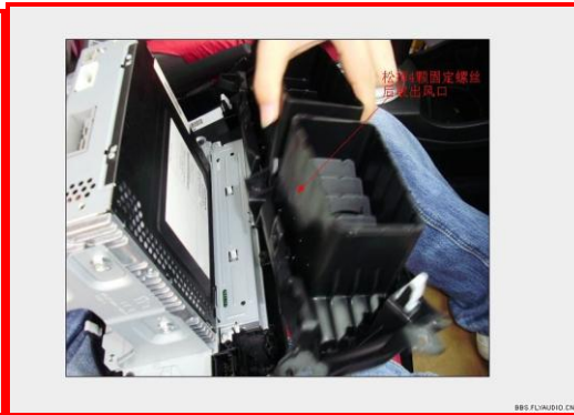
20: install the air letout with FLYAUDIO unit
