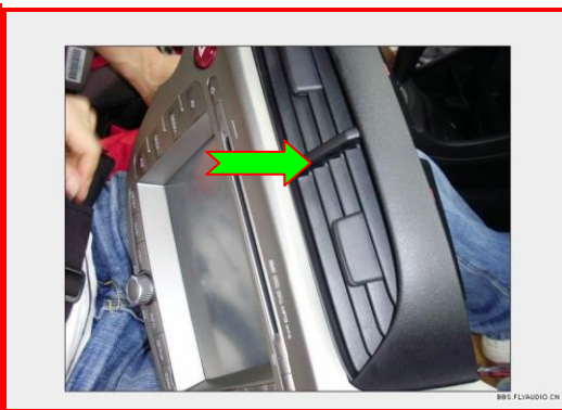
20: install the air letout with FLYAUDIO unit
