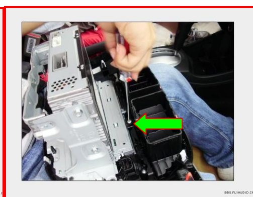
16: Remove the screw of AC
