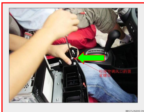
15: Remove the screw of AC
